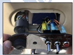
• Note: Connect the small black 2 pin quick connectors that are hanging loose from each switch panel harness. This feeds the backlighting to the port switch panel. They are typically secured to the harness with loose blue painters tape for easy identification.
