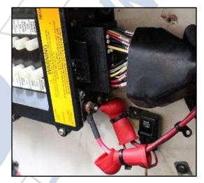
Turn off battery switches and disconnect ALL batteries.
