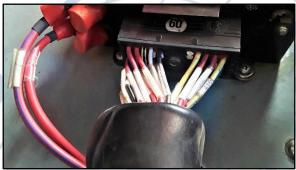
Remove 2 positive (labeled) and 1 negative 8ga cables from the aft EIM box. Refer to the
