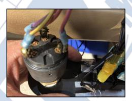
• Note: Connect the small black 2 pin quick connectors that are hanging loose from each switch panel harness. This feeds the backlighting to the port switch panel. They are typically secured to the harness with loose blue painters tape for easy identification.
